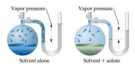
As u see in the picture, when the solvent is pure, the vapor is at the max  $\rightarrow$  the pressure of this vapor is high, but when a nonvolatile solutes is mixed with the solvent, the vapor is decreased  $\rightarrow$  the vapor pressure is decreased.
