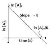
The questions on these diagrams maybe they give u the same diagram with the value of slope & ask for K, or the value of Y intercept & ask for  $\ln [A]_{\circ}$  & so on .
